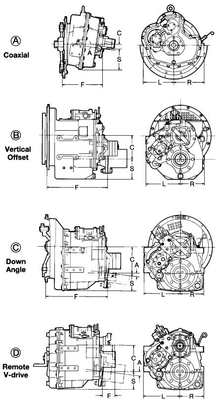
**TWIN DISC MG-300, MG-500, MG-5000 SERIES CONFIGURATIONS**
